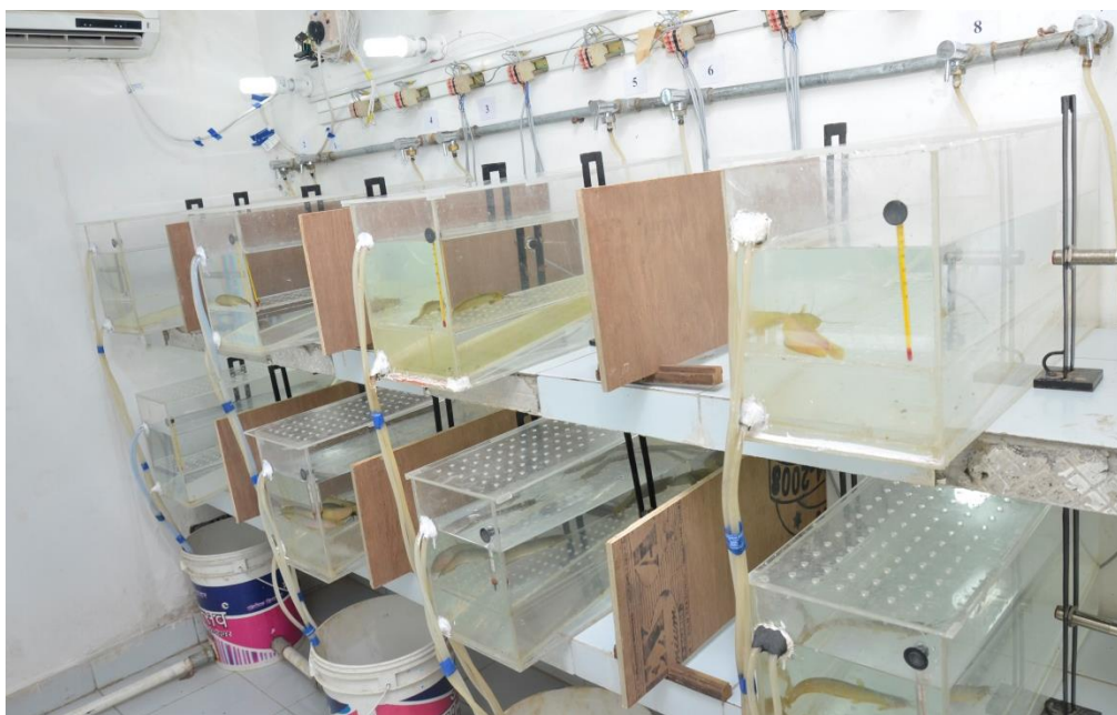
Figure 2. The experimental set up shows eight aquaria placed on two selves. The fishes were housed either in solitary or in a group. Each aquarium is fitted with a thermometer, water replenishment system, and a pair of IR sensors (Tx & Rx).
